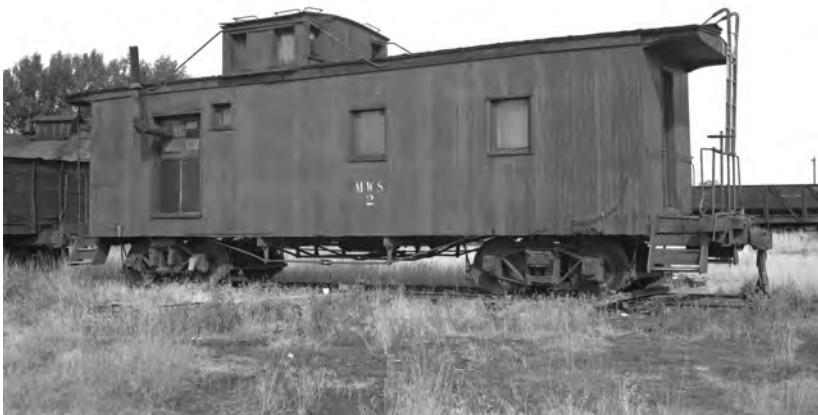
Caboose Number 2 was similar to Number 1 but slightly longer. It is believed to have been built by the YPRR in late 1907. The boarded-up windows and stovepipe extending from the side door suggest that by 1947, it was no longer in revenue service. (Courtesy of California State Railroad Library & Archives).
