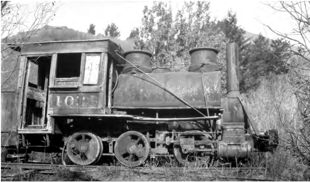
The second locomotive acquired by the Washington and Montana Coal and Development Company was an 0-6-0T. This engine reportedly came from Anaconda's East Helena smelter. Presumed to be an H. K. Porter product, it may have been put to use by the Maxey brothers around 1915. With its drive and connecting rods removed, this 1931 photo finds the engine rusting away near Chestnut. (Museum of the Rockies, RVNo4036, Ron V. Nixon).
