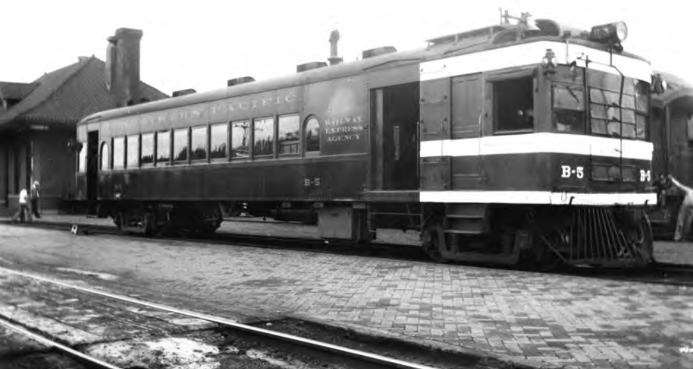
Through passenger service from Bearcreek to Billings was instituted in December 1926 utilizing one of the NP's new EMC gas-electric railcars. Railcar B-5, shown here in Centralia, Washington, in 1936, was the first to be used. An identical unit, B-7, replaced B-5 in 1927 (Emery Roberts Collection [2012.74], Washington State Historical Society, Tacoma).
