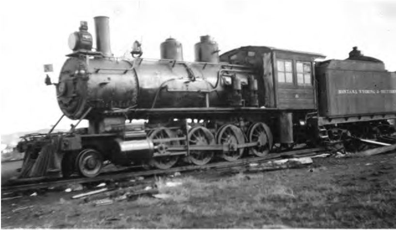
Seen here in Belfry around 1920, consolidation Number 6 was acquired from the Pittsburgh & Lake Erie Railroad in 1916 to help handle the increasing traffic load during the First World War. Note the lack of ballast and the widely spaced ties on this side track in the Belfry yard. (CCHS&M-Kidwell Collection).
