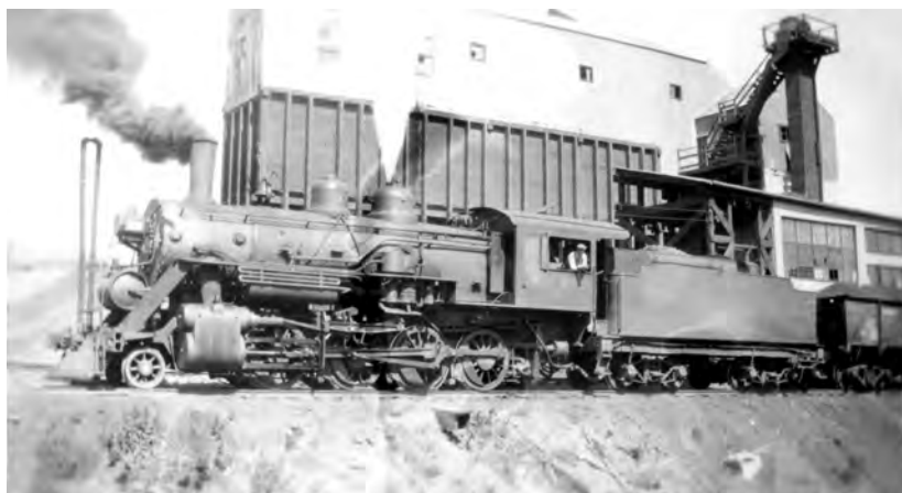
The blast coming from Number 10's safety valve is a sign that the engine has a full head of steam and is ready for the next switching move at Anaconda's no. 2 mine in Washoe. Having done his job well, the fireman can be seen relaxing for a moment while gazing at the photographer. This photo probably dates from the 1930s. (DeGolyer Library, SMU, Everett DeGolyer Jr. Railroad Collection).
