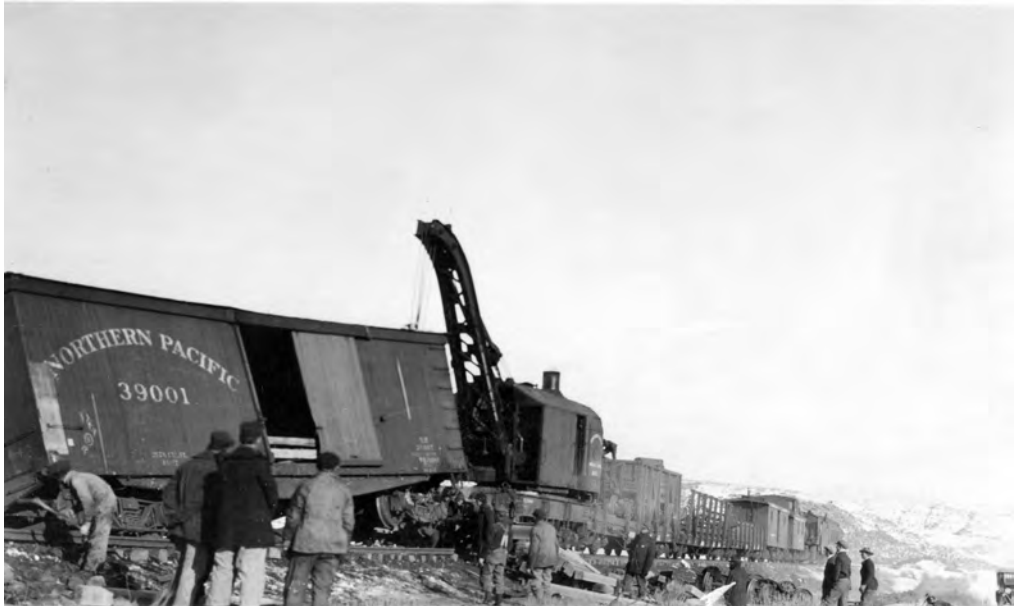
A Northern Pacific work train and wrecker have been hired to clear yet another derailment. Part of a grain door, or slab, is visible in the derailed boxcar's open door. (CCHS&M-Kidwell Collection).
