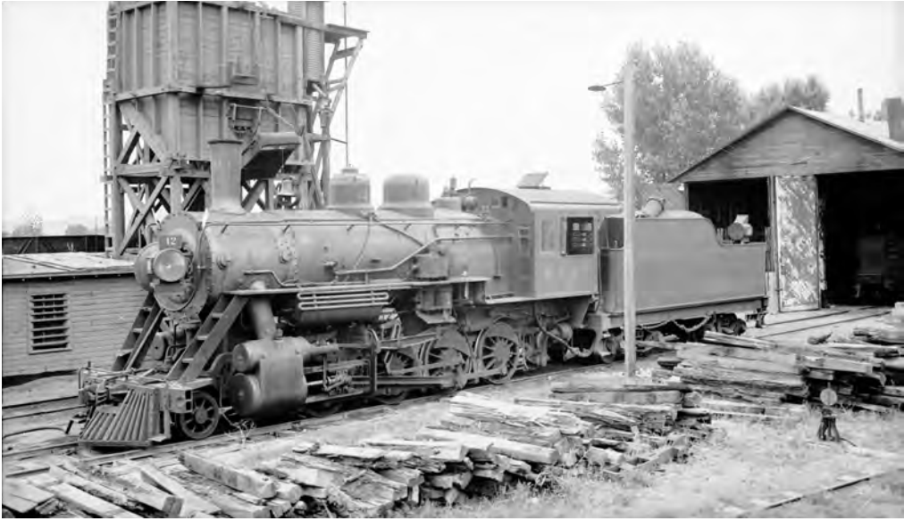
Good photos of Number 12 are rare. In this shot from July 1939, it sits in front of the Belfry engine house with its smokebox door open undergoing light maintenance. The low building on the left houses the winch for the coaling tower. A corrugated metal tank used for locomotive sand can be seen above Number 12's sand dome. (PAC 97-93.02935, MWS 12 Belfry 7/30/39, Montana Historical Society Photograph Archives).
