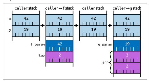
Figure 3-2. Evolution of stack usage as functions are called and returned from
