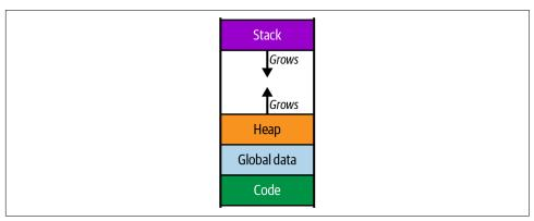
Figure 3-1. Program memory layout, including heap growing up and stack growing down
