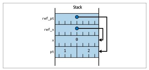
Figure 1-2. Stack layout with pointers to local variables
