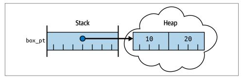
Figure 1-3. Stack Box pointer to struct on heap
