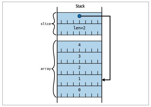
Figure 1-4. Stack slice pointing into a stack array
