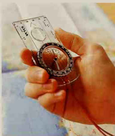
A modern orienteering compass comes equipped with ruled edges and a built-in magnifying glass, together with a rotating rim that allows the orienteer to sight on a landscape feature, set the rim, turn the compass to north and read off the exact angle of the course he or she needs to take.
