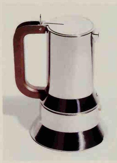
A mocha is composed of two sections separated by a metal filter holding ground coffee. When placed over a stove, the water from the bottom boils into steam, passing through the coffee into the top where it condenses back into water, now infused with caffeine-rich goodness.
