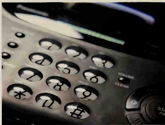
No matter how modern the design, or how advanced the technology, the layout of the telephone keyboard still reflects the original technology of the first number dialing telephones from more than a century ago.
