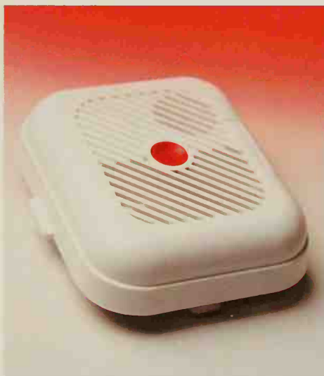
A typical smoke alarm, with a "Test" button in the center. Remember that pressing the button only tests that the battery has not run down and the alarm is sounding properly, not that the detector itself is actually working. To test this, simply direct some smoke or steam into the detector (and cover your ears).
