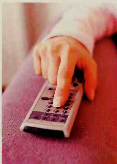
Modern remote controls use infra-red light. Each button has a digital code, and when pressed the remote fires a beam of light carrying that code at the television. The beam is picked up by a photodetector on the TV, which reads the code and triggers an action.
