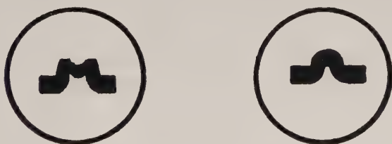
Figure 55: Keyway profiles for wafer tumbler lock.
