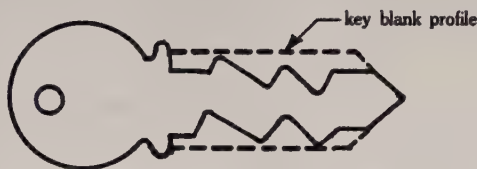
Figure 16: Single wide tumbler key bitting.
