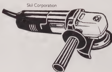
6-9 A disc grinder can be useful for removing high-security screws.
