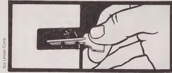
17-31 Hold the key against the face of the spinning brush.
