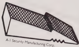
6-28 Wedges are used when opening locked vehicles.
