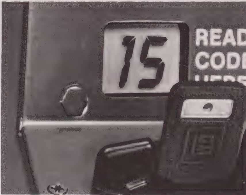
19-7 The resistor value of a VATS key can be determined by inserting the key into the All-Lock A-7000.
