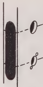
7-26 Drill holes for trim and lock function. Schlage Lock Company
