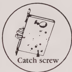
7-30 Install lock case. Schlage Lock Company
