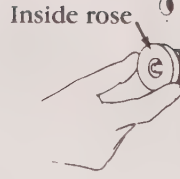
7-33 Install inside lever trim. Schlage Lock Company
