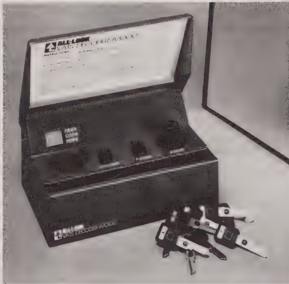
19-6 The All-Lock A-7000 is used to service vehicles with VATS.
