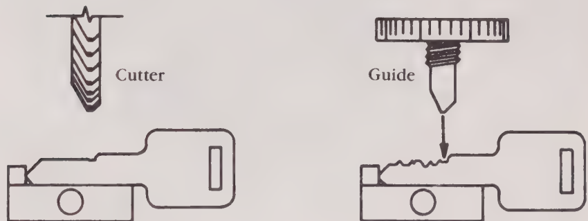
18-16 Set guide in each cut on pattern key. Framon Manufacturing Co., Inc.
