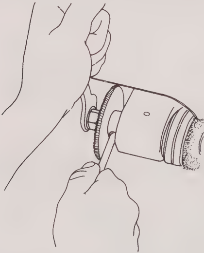
18-7 Insert the stabilizing rod into the hole of the cutter shaft. Ilco Unican Corp
