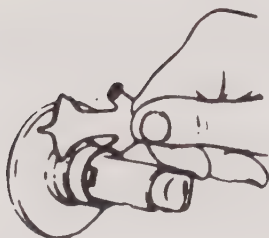
7-12 Use spanner wrench on threaded rose. Schlage Lock Company
