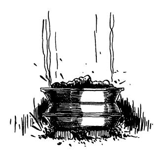
For best results, use heavy gauge, 9-inch aluminum pie pans. Lightweight, alloy pans rust, warp, and don't conduct heat efficiently. Use bolts and wing nuts made of a material that will not melt or shed a coating when heated. I use brass ones and have had good results. I have also seen some steel ones that give satisfactory service.
