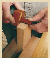
MARKING OUT. A pass with a marking gauge (far left) lays out the depth of the tenon on all four sides; a mortise gauge marks the cheeks (left).
