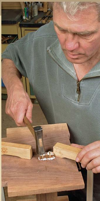
**SOMETIMES CLAMPS ARE NEEDED.** Nesset uses clamps to keep the tenon shoulders snug and square while he drives home the wedges.
