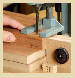
**REMOVE THE SPACER BLOCK** to cut the other end of the mortise. Once both ends of the mortise have been cut, nibble away at the remaining material.
