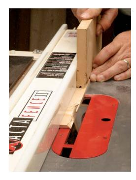
position the workpiece for each cut. I also glue 180-grit sandpaper to the face of the miter gauge to prevent the workpiece from slipping.
