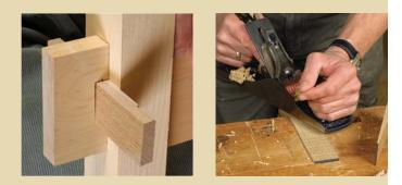
TRY THE FIT, LOOKING FOR GAPS. The wedges may need light planing to adjust their fit in the mortise.
