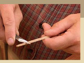
WHITTLE THE PINS. The pins start off square, sized to fit the top of the hole and roughly ½ in. extralong. Then all but the top 1 in. is whittled round (left).
