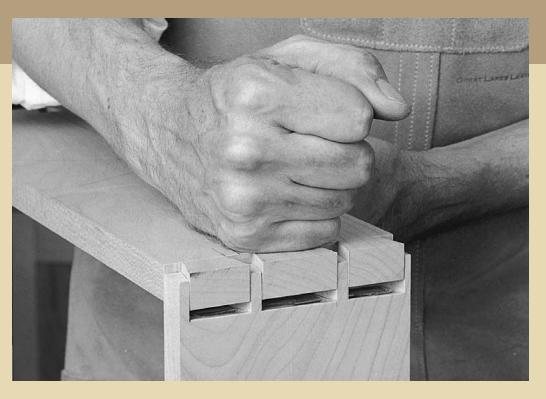
TEST-FIT THE JOINT. If you've cut and pared right up to the lines, the parts should fit like they were made for each other, a snug friction fit that comes together with a light tapping of your fist.
