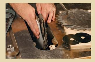
TWO TYPES OF DADO BLADES ARE AVAILABLE. The outside cutters of a stackable set of blades (left) are placed on the arbor first and last, with chipper blades between them. The width of the cut is fine-tuned by placing metal or paper shims between the blades. Adjustable blades (below), also called wobble blades, can be adjusted to width by rotating a dial on the side of the blade.
