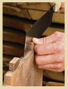
SAW A KERF DOWN TO THE HOLE. A handsaw leaves an appropriately narrow kerf in the tenon.
