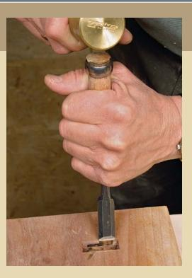
LAY OUT THE OFFSET of the angled mortise. After determining the offset at the top of the mortise, scribe lines to indicate where the angled cuts begin (left). Work steadily back toward the scribe line (above) and down toward the bottom edge of the mortise.
