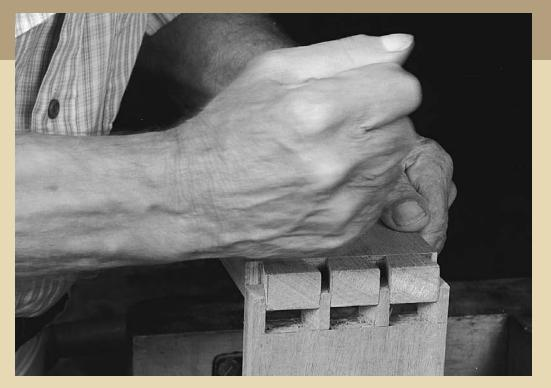
CHECK THE FIT, make any necessary corrections and tap the joint closed. It should go together with a light tap of your hand. Don't forget that the joint will swell when you apply the glue.
