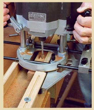
**STEADY AS SHE GOES.** The router base sits firmly on the top of this jig as the router fence indexes the location of the mortise.
