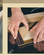
TO SET THE MITER GAUGE AT EXACTLY 45°, first align a drafting triangle against the miter slot in the tablesaw (left). Make a cut in a piece of scrapwood (center). Flip over the cutoff piece and hold both pieces tightly against a square (right). Adjust the miter gauge until there is no gap, and you are set to cut perfect miters.
