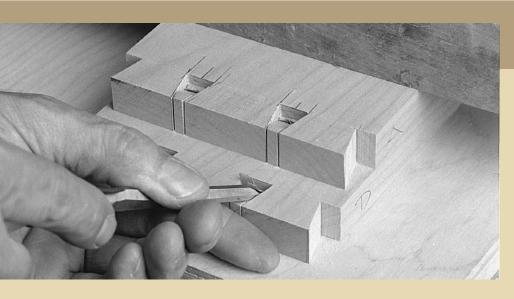
CHOP OUT THE WASTE. Start by creating a small groove on the waste side of the baseline. Then chop alternately in at a sharp angle (above) and downward at a slight angle (right). Don't chop in from the end of the board yet. Keeping the corner intact prevents tearout when the waste is removed from the center of the socket. Once you've chopped about halfway through the joint, flip the boards over and repeat. This time, though, chop from the end.
