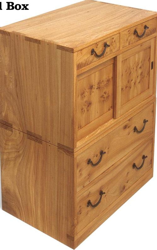
**B** oxes are the essential structure of all case pieces. That means a large part of furniture making boils down to joining pieces of wood to make boxes. There are many ways of doing this. Some, such as dovetails, draw attention to the joinery and the box structure itself, while others, such as post-and-panel construction, hide those aspects.
