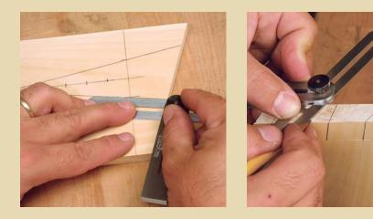
TAKE THE TWO SETTINGS from the layout board. Lay out one of the angles on all of the pins or tails, then reset your bevel gauge to the other angle and finish the layout.
