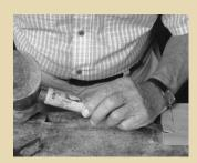
ALTERNATE CHOPPING from the face of the board and the end. When chopping on the face, hold the chisel in at a slight angle so that the tail slot is undercut. Chop just about halfway through the board. Flip the board over and repeat.
