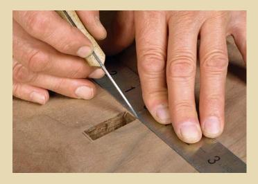
ANGLE THE ENDS OF THE MORTISE. The layout and chopping techniques are the same as when angling a mortise for a single fixed wedge.
