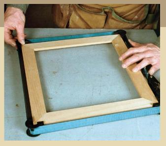
A BETTER BAND CLAMP. Plastic corner blocks added to a band clamp reduce the risk of crushing the corners of the workpiece.
