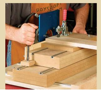
ADJUST MORTISE DEPTH ON THE ROUTER. The distance from the fence to the end of the router bit determines the depth of the mortise (top left).
