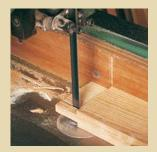
A BANDSAW TRIMS THE CHEEK. With the fence set in place, a quick pass cuts to the shoulder line. After adjusting the fence, another cut establishes the top and bottom of the tenon. A backsaw and chisel are used to clean up the shoulders.
