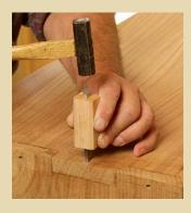
SHOPMADE TOOL for squaring holes. Janofsky uses a thin, square bar of steel, tapered on a bench grinder, to square the holes. The wood block makes the tool easier to hold.
