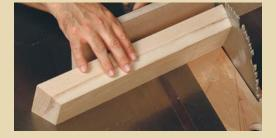
HOLD THE BLOCK IN PLACE and bring up the miter gauge. When the gauge is flush to the block, lock in the angle setting.
