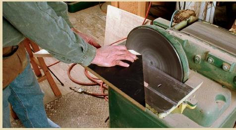
SAND TO FIT. Another way to fine-tune a miter joint is to use a jig that holds the workpiece at 45° to a sanding disc.
