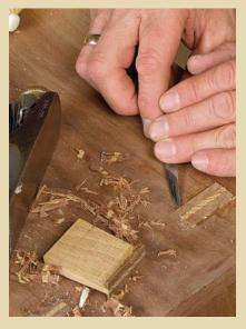
A TRICK FOR A CLEAN, FLUSH JOINT. To prevent tearout when planing a tenon flush, score a line around the base of the tenon.
