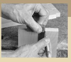
MARK OUT THE PINS from the tail board. Clamp the pin board into a vise, and set the tail board perpendicular to it. Make sure the edges of both boards are flush, and be sure the inside edges of all the sockets align perfectly with the inside corner of the upright board. Apply pressure to the top board, and mark the dovetails with a sharp knife (far left). Extend the pin marks down the side of the pin board using a small square. Cut down to the baseline on the waste side of the line.
