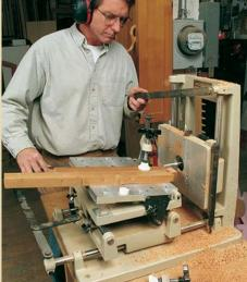
**ROUTING MACHINES** for production work. Guided by templates or set by hand, the horizontal routing machine takes a little work to set up but can cut countless tenons in no time at all. The table also tilts to make easy work of angled tenons.
