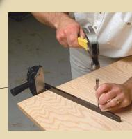
A TIGHTER FIT. If your miter gauge has some side-to-side slop in the miter slot, punch the edge of the gauge bar with a center punch. This spreads out the metal to tighten the fit.
