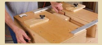
**BUILT-IN VISE HOLDS THE WORKPIECE IN PLACE.** The crank (at left in photo) controls a plywood box that pushes against the workpiece to hold it secure. The top surface of the workpiece should be flush with the top of the plywood table.
