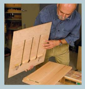
**ROUTER TEMPLATE SPACES PARTITIONS EVENLY.** Because the stopped dadoes for the partitions must be cut precisely and in identical positions on both the upper shelf and the top, it is best to use a plywood template to guide the router.
