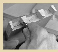
**CHOP OUT WASTE BETWEEN PINS.** Clamp the boards so their inside faces are up (left). This prevents the chips from becoming wedged between the pins when you finish chopping out the waste from the other side. When you're about halfway through, turn the boards over and re-clamp (center). As with the tail boards, once you've flipped the boards over, you can chop in from the end. Pare to the line with a chisel (right).
