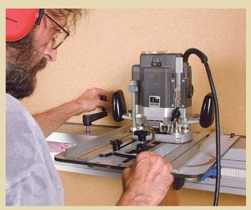
CLIMB CUTS ARE CLEANER. You can virtually solve the problem of chipout on the leading edge of the router cut by moving the workpiece in a clockwise direction around the cutter.
