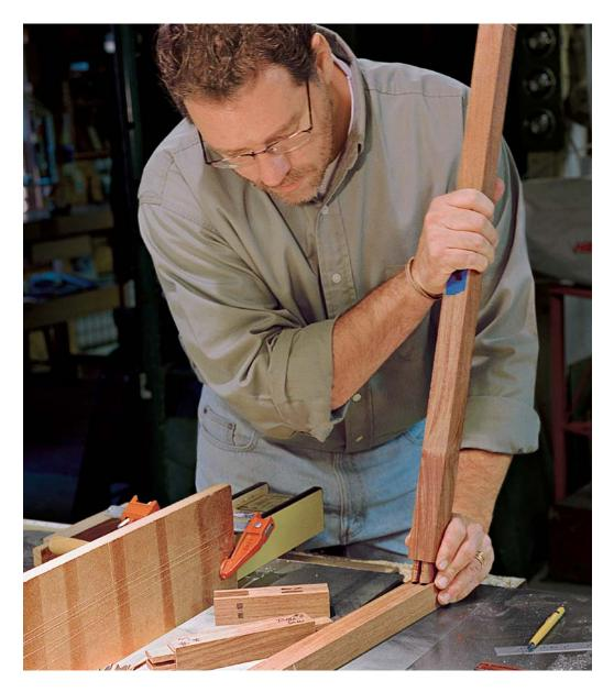
TOOLS FOR MULTIPLE MARKING. A story stick and a marking knife add accuracy and reliability to a repetitive process.
