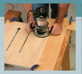
CUT THE TEMPLATE GUIDE. With a T-square guide clamped to the edge of the plywood template, rout a slot for the template guide to ride in.
