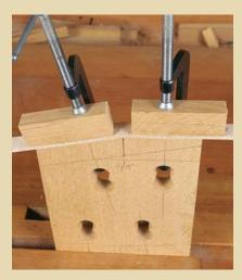
TEST TENON STRIP MATE-RIAL WITH A TEMPLATE. A few outside fibers have failed on this test strip, but it is basically sound.
