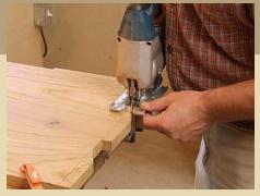
SAW THE CHEEKS and chop out most of the waste. Janofsky uses a Japanese dovetail saw (left), which cuts on the pull stroke and should be held at the end of its handle for the best results. Cut right to the layout lines, being careful to keep the cut straight and square. Use a bandsaw or jigsaw (above) to remove most of the waste.
