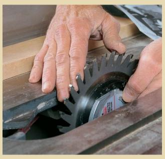
raising the dado blades through the insert to a predetermined height. Instead of starting and stopping the saw to measure the blade height, I mark the depth of cut on my rip fence and slowly raise the blade to that mark.
