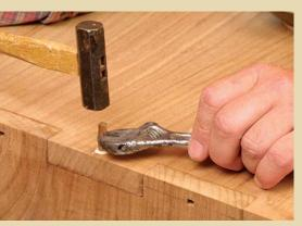
**DRIVE HOME THE PINS.** Add give to the pin and hole, and drive in each pin while holding it in alignment with a wrench.
