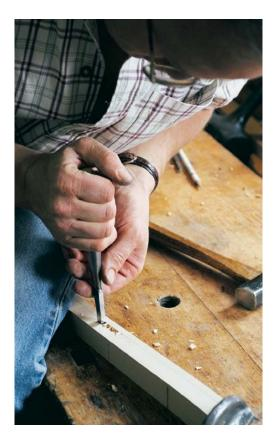
MAN OR MACHINE. Everyone can find a way to cut mortises well, whether through improving skills or finding a better tool. Some prefer the quiet approach of the chisel (above), and others go for the fast and furious router (right). Other good options include the drill-press-and-chisel approach, hollow-chisel-mortise machines and dedicated slot mortisers.
