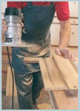
SHOPMADE T-FENCE FOR CUTTING DADOES. Screw two strips of plywood together at right angles to make a guide fence for cutting dadoes with a router.
