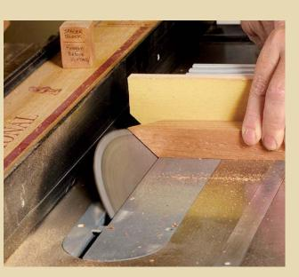
**ROTATE THE WORKPIECE** to cut the adjacent miter. The mortise that was facing the surface of the tablesaw should be facing the miter gauge on the second cut.
