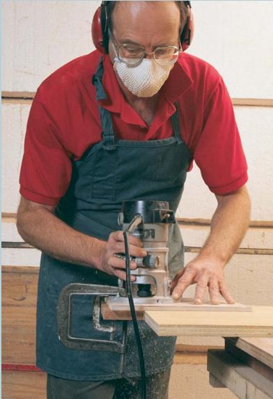
A BLOCK OF WOOD and two clamps make a fence. An auxiliary fence helps create a clean rabbet by spanning dips that a bearing would follow.
