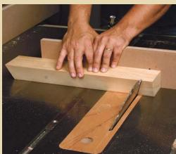
NOW MAKE THE SET-UP BLOCK. Mill a flat, square block roughly 2 in. thick by 3 in. wide by 10 in. long. Then rip one edge (left) and crosscut the two ends at the slope angle (above).
