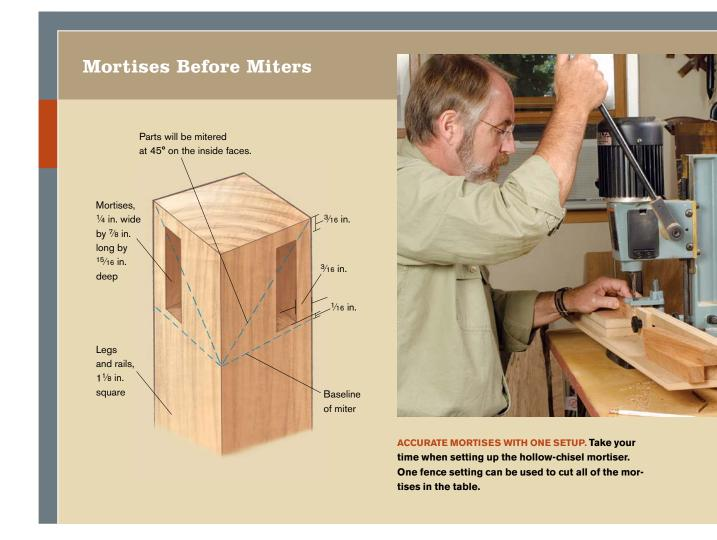
method in which all of the mortises are cut with one fence setting on a hollow-chisel mortiser; all of the miters are cut with one setting on the tablesaw; and loose tenons are used to join the pieces. Furthermore, the four rails and four legs that make up the basic table are all produced with the same series of cuts.
