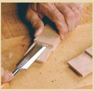
all the pieces. FINE-TUNE THE FIT. Rasps and chisels are good
