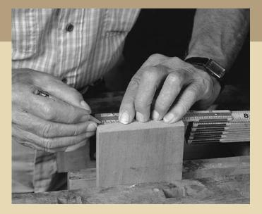
MARK PINS AND HALF PINS on the end of the board. You can space them by eye, or use a ruler for more consistent spacing. A pencil mark is plenty accurate at this stage, because the pins are the first parts of the joint to be cut.
