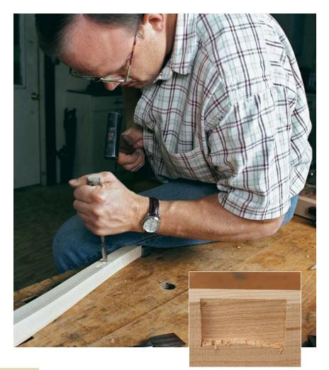
smooth-but-unburnished surface, free of loose fibers, because glue needs to penetrate a few thousandths of an inch into intact wood. If the surface is burnished—by a dull router bit, for example—the glue can't seep into the pores and has little grip. If the surface is covered with loose fibers, such as a dull chisel might leave, the glue attaches to the loose fibers and not the joint walls. The lesson here is that sharp tools increase joint strength.
