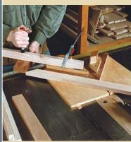
LENGTH. Mark the length on the workpiece and on the right-hand fence. Clamp a stop block against the mitered end.
