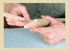
**SIZING THE JOINT.** The open grain on the face of a miter should be sealed with a thin layer of glue and allowed nearly to dry. The sealed end grain won't starve the joint when glue is applied to connect the miter.
