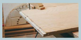
**ROUTER BITS WITH BEARINGS HAVE LIMITATIONS.** A bearingpiloted bit (top photo) will dip into voids and round corners. The result is a sloppy rabbet (bottom photo).
