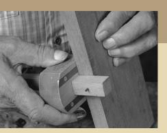
**SET THE MARKING GAUGE** <sup>1</sup>/64 IN. WIDER than the stock, so the pins and tails will protrude slightly.
