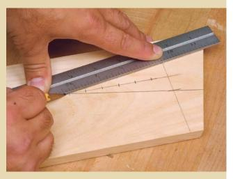
MARK OUT SIX DIVISIONS of the same thickness as the sides to create a 6:1 dovetail angle. Use those lines to set your sliding bevel gauge. There will be different gauge settings for the tops and bottoms of the pins.
