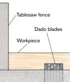
CUTTING A DADO. the depth of the dado should equal about a third of the wood's thickness. Apply constant pressure both against the fence and downward to ensure that the cut is consistent in depth across the piece. With narrow workpieces, use a miter gauge for guidance and support.
