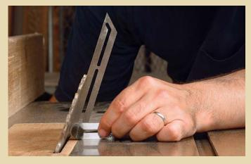
**TRANSFER THAT ANGLE TO THE BLADE.** This is a good time to rip the top and bottom edges of the box sides, which usually are cut at this angle.
