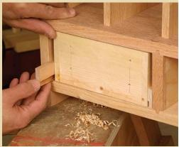
**DRAWER GUIDES** have a rabbet and stop  $1\frac{1}{2}$  in. from the back slats. This allows the thickness to be trimmed with a block plane after they have been installed.
