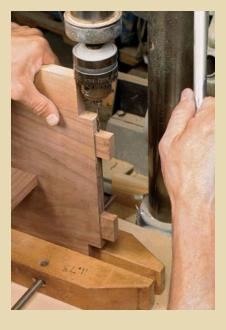
DRILL A HOLE to prevent the tenon from splitting. Clamp the workpiece vertically in a handscrew. Then drill a hole through the width of the tenon.
