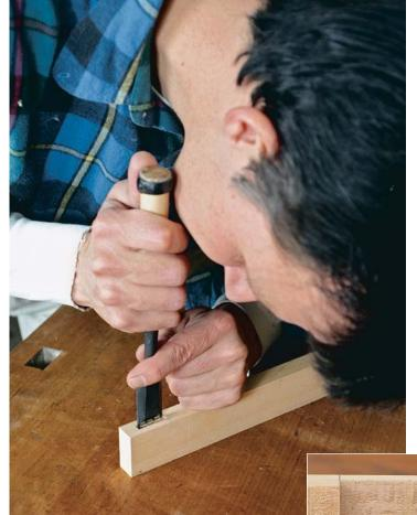
a well-tuned mortising chisel is almost selfguiding after the first <sup>1</sup>/<sub>6</sub> in.
