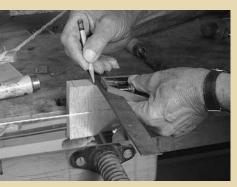
MARK THE TAILS from the pins. Hold the pin board securely in place on the tail board. The edges of both boards should be flush with each other and the inside face of the pin board should rest on the baseline of the tail board. Scribe the tail layout from the inside of the joint so that the awl follows the pins, not the grain. Extend the marks across the end of the tail board. Then cut the tails down to the baseline. A mirror makes the layout lines easier to see. Split the line on the waste side.
