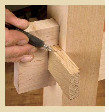
is inserted from one side and one from the other, and both are driven in until the two angled faces lock. Orientation is horizontal instead of vertical because the bottom wedge would work loose and fall out in a vertical configuration. With each edge of the wedges and the edges of their mortise neatly chamfered, the double wedge makes a useful, strong, and attractive joint.
