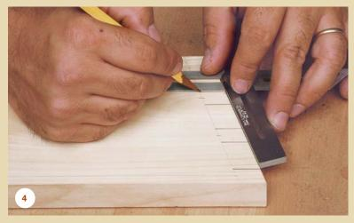
a square, keeping the line parallel to the beveled edge and the blade of the square flat on that edge. Last, use a straightedge to carry the shoulder line across the other face.
