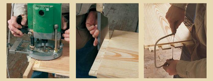
AN EDGE GUIDE helps rout tenons on wide boards. When cutting breadboard ends or fitting a headboard to bedposts, wide tenons can be a beast to cut. A router with an edge guide (or registered against a temporary fence) does the job in a few passes (left). After the shoulder has been established, a backsaw and coping saw rough out notches to allow for wood movement (center), and a final pass with the router evens out the notch (right).
