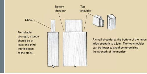
the tenon has been fine-tuned with a rabbet or bullnose plane, use the same methods to cut any haunches or other shoulders. Then grab a chisel and a plane to help you fit the tenon exactly to the mortise, trimming only a little at a time and test-fitting frequently.
