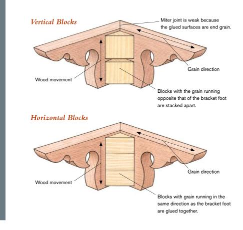
grain legs, as in the butternut chest on p. 45, are only slightly stronger because the glue surfaces of the miters are long grain.
