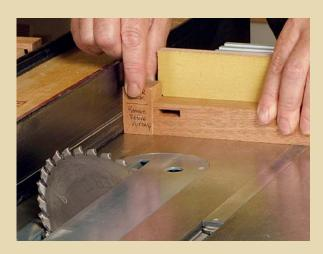
BUTT THE WORKPIECE against a stop block. Position the stop block so that the sawblade cuts right to the corner of the workpiece. Be sure you don't cut past the corner line. The first miter is cut with the workpiece held so that one mortise is facing the blade and the other is facing the surface of the tablesaw.
