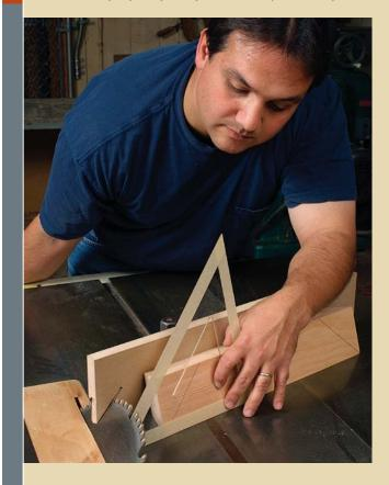
PLACE THE TRIANGLE FLAT against the front face of the set-up block. Angle the blade to meet the edge of the triangle.
