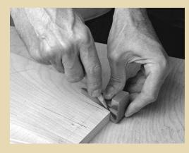
MARK THE ANGLES of the pin sockets with a dovetail gauge or a bevel square. Transfer these lines across the end grain. Now tape the two tail boards together, so you can cut pin sockets on both at the same time.
