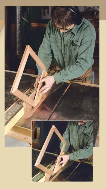
**ONE JIG CUTS TWO KEYS.** Simply by adjusting the fence of the tablesaw, the key-cutting jig can cut either straight keys in the center of the frame (photo above), or face keys on the front of the frame (inset).
