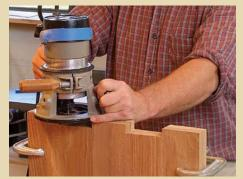
TALL PIECES ARE EASIER to handle with a router. Clamp pieces in pairs to give the router a wider bearing surface. Set the bit depth right to the scribe mark.
