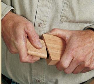
LOOSE TENONS FOR LONG STOCK. Sometimes lengthy boards are difficult to muscle around machines, but using loose tenons is a simple solution. A mortising template (left) guides a bearing-guided straight bit to cut mortises in both pieces you're trying to join. Tenon stock is cut to width and thickness, then the long edges are rounded (top photo) to fit the mortise. Short sections are trimmed to length and glued in place (above).
