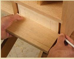
FIT THE DRAWER FRONTS. After cutting the false fronts to size, mark the location of the drawer box on the back of each, including the holes. To attach the drawer front, drill the holes in the drawer box slightly oversize to allow for fine-tuning to the opening.
