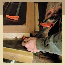
NO BAND CLAMPS HERE. Because the spline extends beyond the outside corner, it is necessary to use block clamps.
