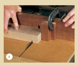
MAKING THE SHOULDER CUT. With a stop block clamped in place, a quick pass with a crosscut sled cuts the tenon shoulders (1). After a bandsaw hogs off the cheek waste, a tenoning jig-shopmade or aftermarket-holds the stock vertically to fine-tune the cut (2). Another pass with the crosscut jig cuts the top and bottom shoulder and any haunch (3).
