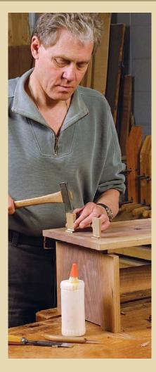
A WEDGE MUST PUSH THE TENON against the end grain of the mortised piece to avoid splitting the wood. So the orientation of the tenon-along the grain or across the grain-determines the number and orientation of the wedges.
