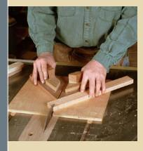
1. THE FIRST CUT IS MADE on the left-hand side of the jig. If the work slips, it will do so away from the blade.
