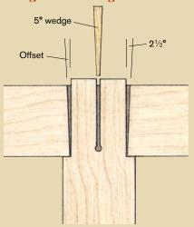
A 5° wedge requires each face of the mortise to be angled at  $2^{1/2}$ °. Draw a cross section of the joint to determine the amount of offset at the top of the mortise.
