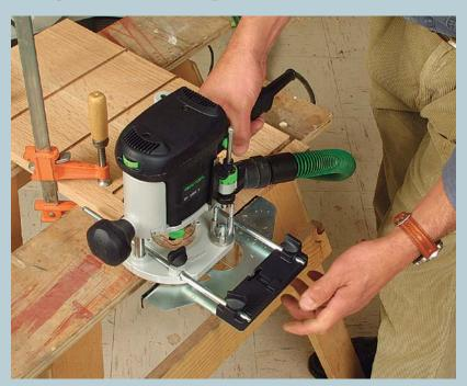
AFTER CUTTING THE STOPPED DADOES for the partitions, add an adjustable fence to the router and cut the stopped dadoes at both ends of the top to receive the sides.
