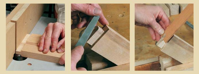
GANGING UP ON THE ROUTER TABLE. A router table allows you to gang up two or more boards, making fast work of cutting uniform tenons (left). If the mortises are cut with a router as well, the author uses chisels and files to round the tenon (center), checking his progress with a template routed to match the top and bottom of the mortise (right).
