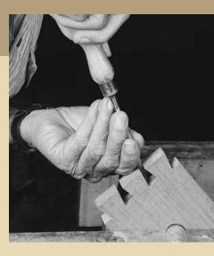
WITH AN AWL, connect the baselines from both sides of the board (left). Chop away the waste between the tails, first creating a little bevel to prevent tearout at the baseline. Alternate chopping from the end and face until you're halfway through the board (center). Then flip it over and repeat. Clean out the corners (right). The little bit of wood remaining at the base of the tails often prevents dovetails from closing.
