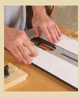
ADJUST THE PLATE TO CEN-TER THE CUT. The phenolic plate rides left to right on four loose bearings that rest on the plywood tabletop and is held in place by the two aluminum bars on both ends.
