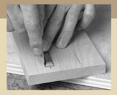
USE A CHISEL to determine the width of the pin sockets. This makes chopping the sockets much more efficient. Place the chisel over the centerline, and use a pencil to mark each side. Then mark out the half-pin sockets on the ends.
