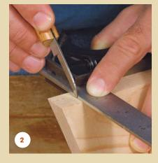
2. CARRY THE LINES ACROSS THE EDGES. Using a square with its blade laid flat along the beveled edge of the workpiece, scribe the lines with a knife.
