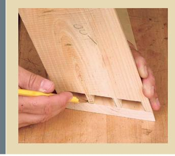
CUT THE PINS OR TAILS and transfer their locations to the mating board. It's no easy feat to keep these angled boards in perfect position during this step.
