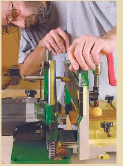
LOCATE THE TENON CUT. Vertical adjustments in the yoke assembly will affect where a tenon is cut on the workpiece. The steel stylus shown here is mounted at a fixed distance from the cutter, and you can use either the small or large end of the stylus to follow the template, which affects the size of the cut.
