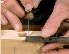
ANOTHER METHOD for laying out the mortise angle. First chop a square mortise through the tenon and make the wedge stock. Insert the wedge and measure the gap at the loose end. That gap is the same amount that the mortise must be offset to match the wedge angle.
