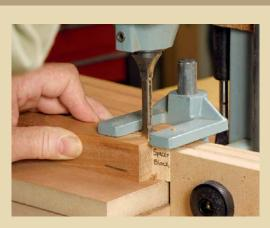
CUT ONE END of the mortise on each piece. With the stop block and fence set on the hollow-chisel mortiser, use a spacer block to guide the first cut for the mortise.
