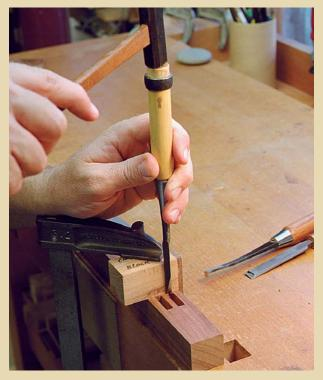
HELP WITH THE HANDWORK. A thick block of wood clamped firmly to the workpiece serves as a guide to chisel the ends of the mortises true and square.
