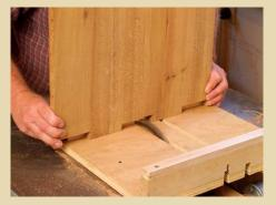
A TABLESAW SLED will handle shorter pieces. Adjust a dado set to cut to the scribe line. Use a sacrificial fence to minimize chipout on the back side of the cut.
