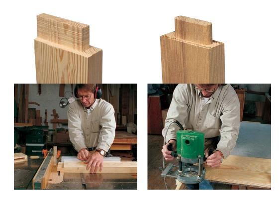
Hand-cut tenons require careful setup and layout (see the photos on p. 84). Your method may involve using a marking gauge and square, a mortising gauge or a pencil and square. But whatever your method, be consistent with your approach and always be dead-on accurate. Even if you are using machines to cut tenons, the same guidelines for marking out hold true.
