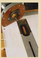
ROUND OR SQUARE TEN-ONS. By varying the shape of the adjustable inserts in the phenolic plate, you can cut either round or square tenons.
