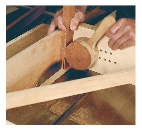
To test the tenon setup, cut the cheeks first. The height of the sawblade off the table does not change. One pass per side is
