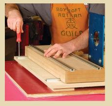
THE MOVABLE PLATFORMS don't make contact with one another; instead, they slide solely on the aluminum T-tracks. The tracks also secure the clamping blocks. Wax the tracks regularly to ensure smooth movement.
