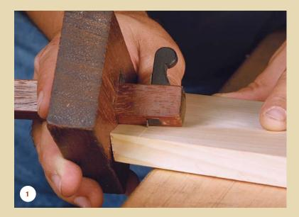
**1. USE THE MARKING GAUGE** on the inside face (with the sharper edge). Rub the beam along the face of the board to keep the gauge in proper alignment.
