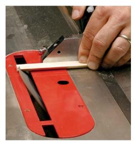
saw or miter saw. Continue the process of mitering the ends and then chopping them to size until all 12 tenons have been cut. Cutting small pieces with power tools generally is a dangerous process, so use extreme caution.
