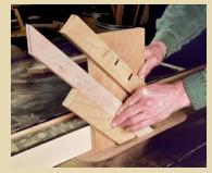
**CUT ONE END.** Hold the workpiece firmly in place and register the jig against the tablesaw fence.
