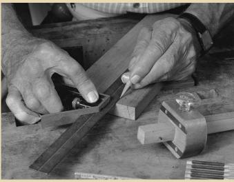
EXTEND THE PIN MARKS down to the baseline using a combination or try square.
