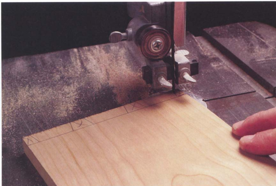
Photo C: I rough cut the tails on a band-saw. Afterward, I use a chisel to pare to the cut lines.
