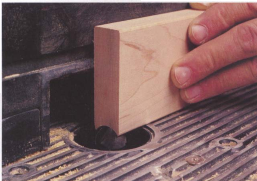
Photo F: Rout the cove in the pawl assembly using a \frac{3}{8} -in.-diameter corebox bit in a router table. The cove accommodates the wooden hinge dowel in the ratchet mechanism.
