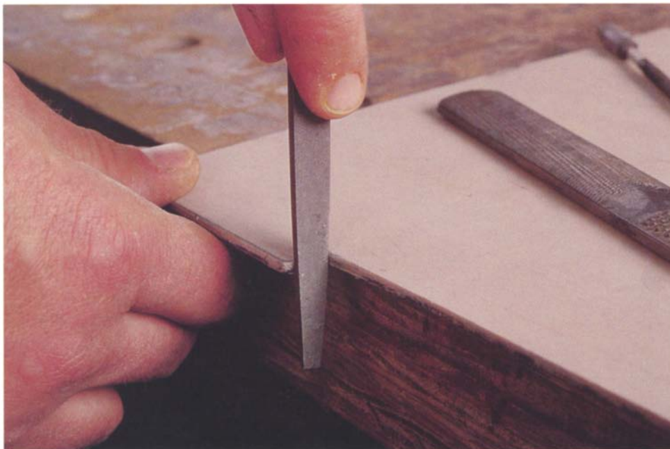
Photo B: Smooth the edge of the template using a combination of files, rasps, and sandpaper.
