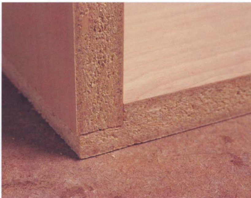
A rabbet joint is a butt joint that is restrained on one side by a ledge, called a rabbet, that is cut into the mating piece. The joint is not as strong as a dado joint and is often reinforced with screws, nails, or other mechanical fasteners.
