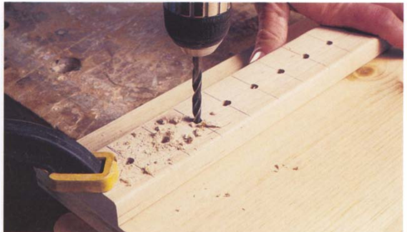
Photo G: A scrap board with guide holes is handy for drilling holes in case sides for adjustable shelves.
