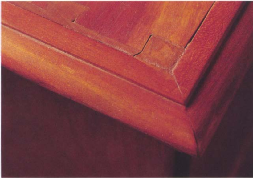
Wood expands and contracts across the grain only. The molding on this case was glued cross-grain to the dovetailed case side, creating a crack as the case side shrank.
