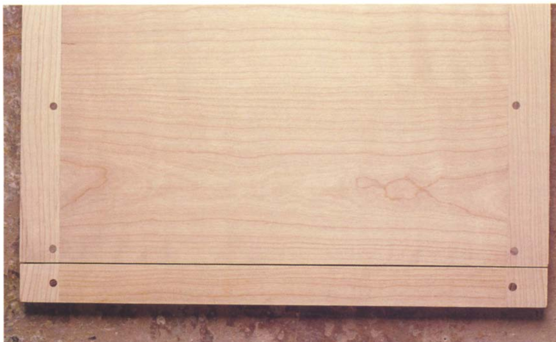
Photo G: Notice how the grain pattern is continuous between the lid and top and the breadboard ends.
