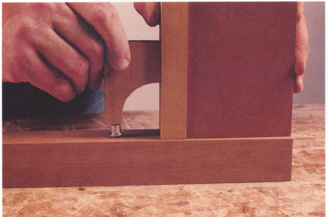
Photo J: Place the bracket assembly against the bottom rail with a dowel center in the tail hole. (The dowel center shown here actually slips over the dowel itself.) Then press the assembly against the leg to locate the mating dowel hole.
