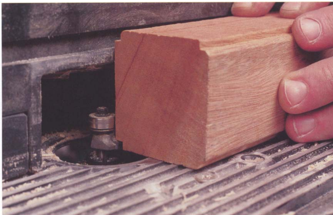
Photo E: Ease the edges of the leg rabbets with a \frac{1}{8} -in.-radius roundover bit.
