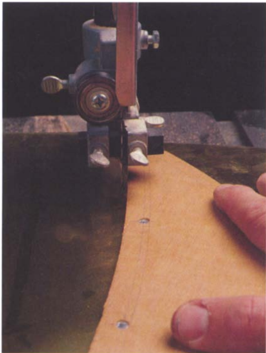
Photo 1: To cleanly bandsaw the brass scuff plate, you can keep it from flexing by sandwiching it between an upper plywood template and a backup scrap piece.
