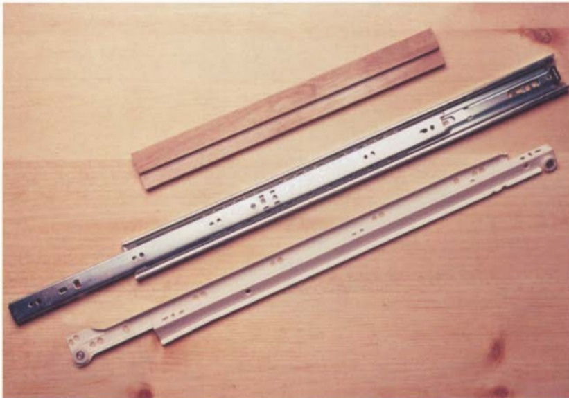
A drawer slide may be made out of wood or metal. The unpainted metal slide shown here mounts at any height on the side of a drawer. The white one mounts on the bottom edge of the drawer side.
