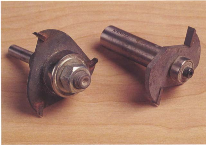
Photo D: A slot-cutting bit is a quick way to rout the mortises for the exposed splines.
