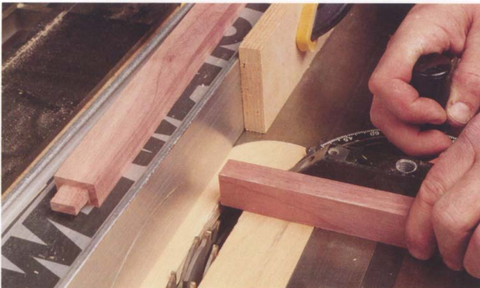
Photo B: A dado cutter in a table saw works well for sawing tenons on short pieces.
