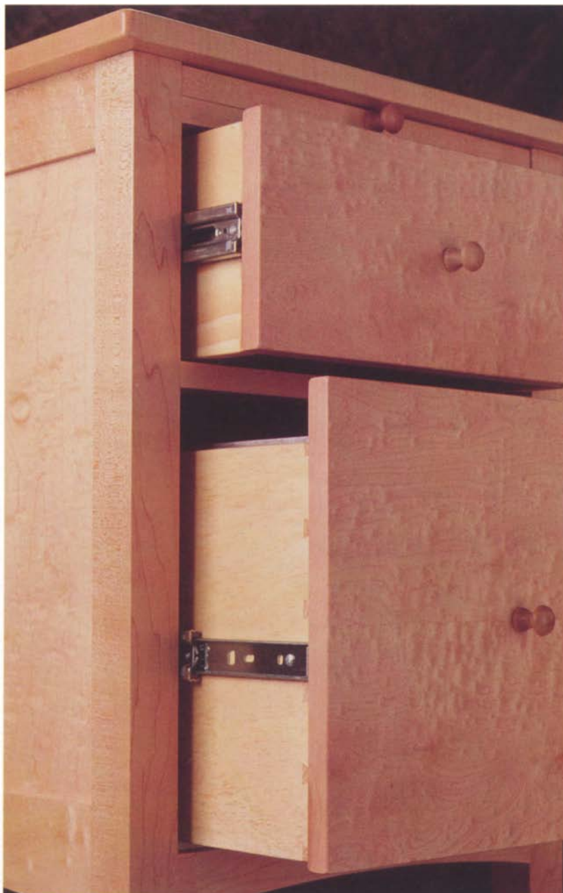
Photo F: The drawers are installed with commercially made, side-mounted drawer slides.
