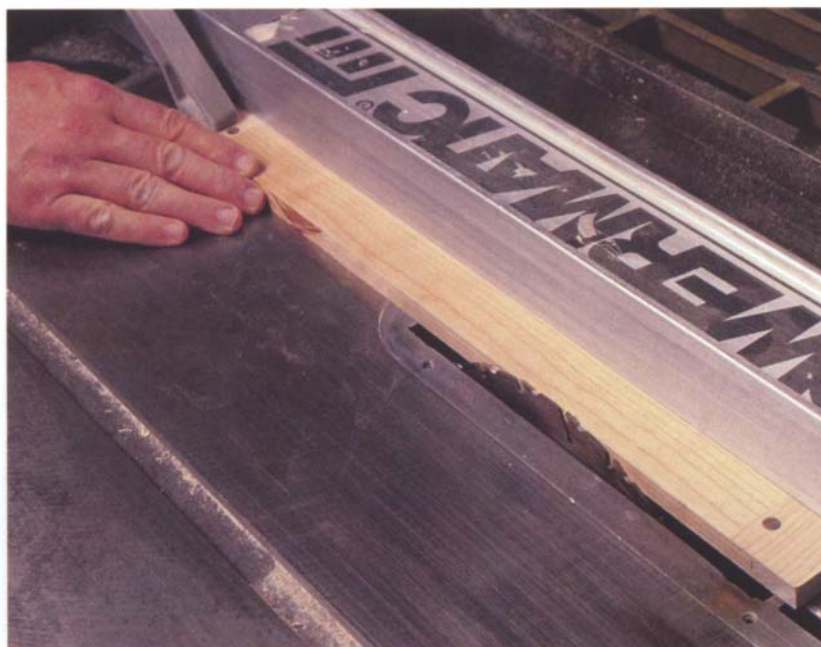
Photo H: After sawing the rail from the top assembly, cut a 5-degree bevel along its front edge.
