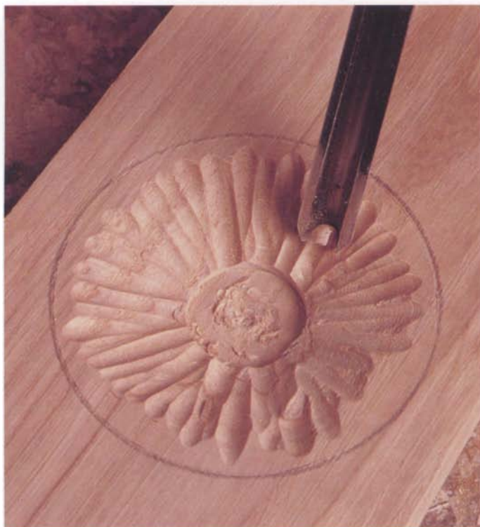
Photo J: Rough out the recess with a gouge, carving from the perimeter inward.
