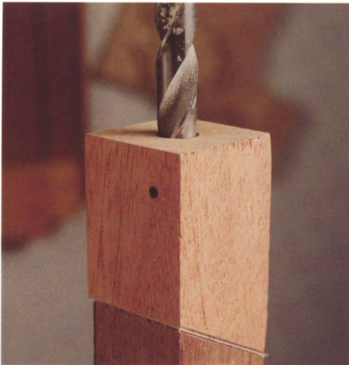
Photo I: To drill the dowel holes in the legs, use a jig that is cut to a complementary angle to that of the legs. Sandpaper on the face of the jig helps keep it in place when drilling.
