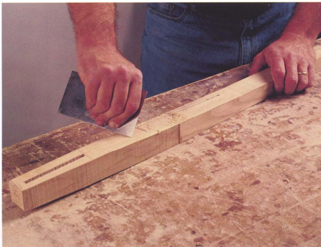
Photo E: I use a scraper to smooth the saw marks from the bandsawn leg.
