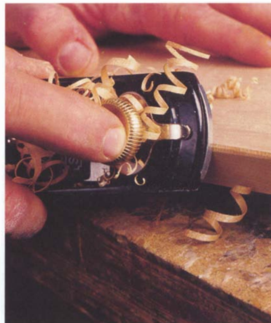
Photo B: After sawing the bevels on the edges of the top, smooth the cut and round the edges using a block plane.
