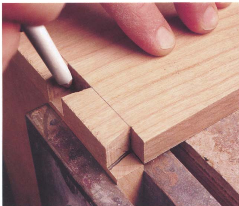
Photo D: I lay out the pins by tracing around the tails.
