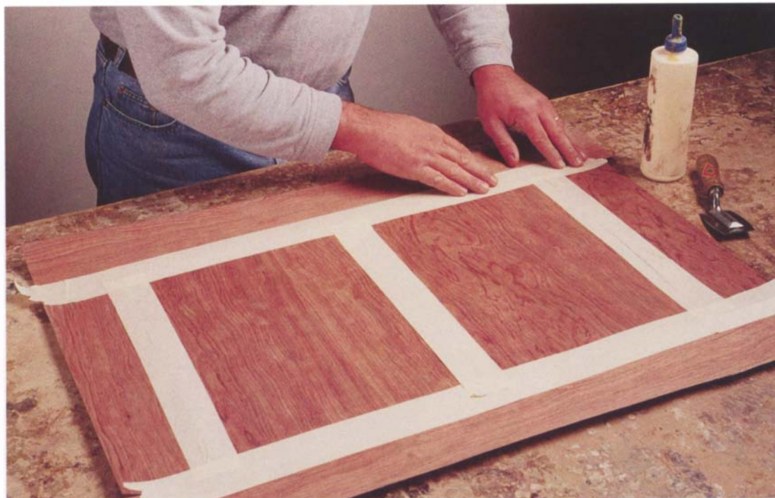
Photo G: Before applying a composition of veneers to a substrate, glue the pieces together at their edges, holding them in place with tape placed on the show side of the veneers.
