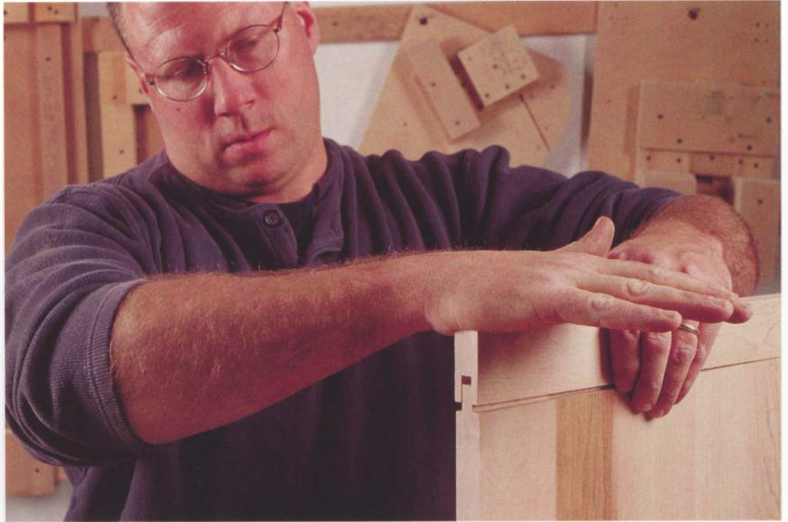
Photo I: The tongue on each end of the pull-out board should fit snugly into the groove on the breadboard end, but not so tightly that you have to pound it in with a hammer.
