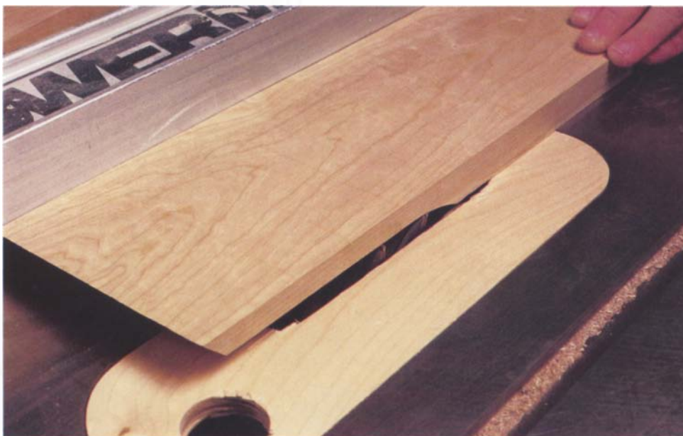
Photo C: Saw a rabbet in the top edges of the case sides and front to recess and support the case top.
