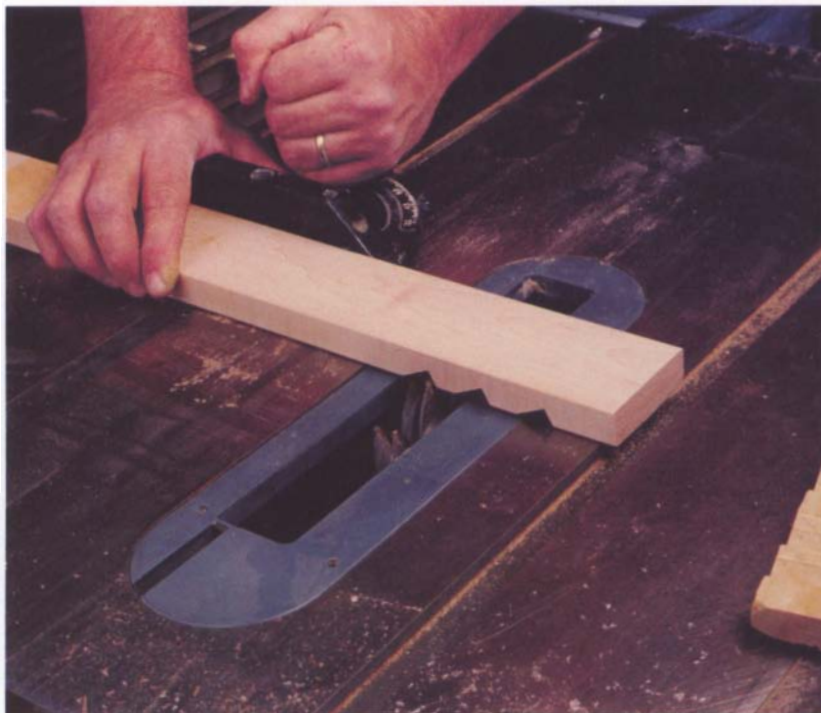
Photo H: Cut the notches in the ratchet bars using a \frac{3}{4} -in.-wide stack dado tilted 30 degrees on the table saw.
