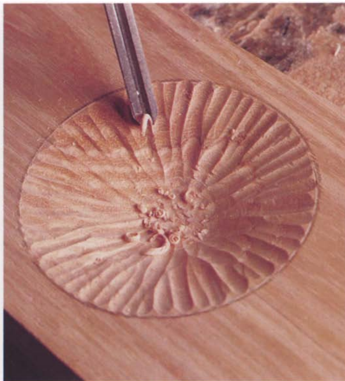
Photo K: Use a veining tool to texture the recess, spacing the cuts evenly around the circle.
