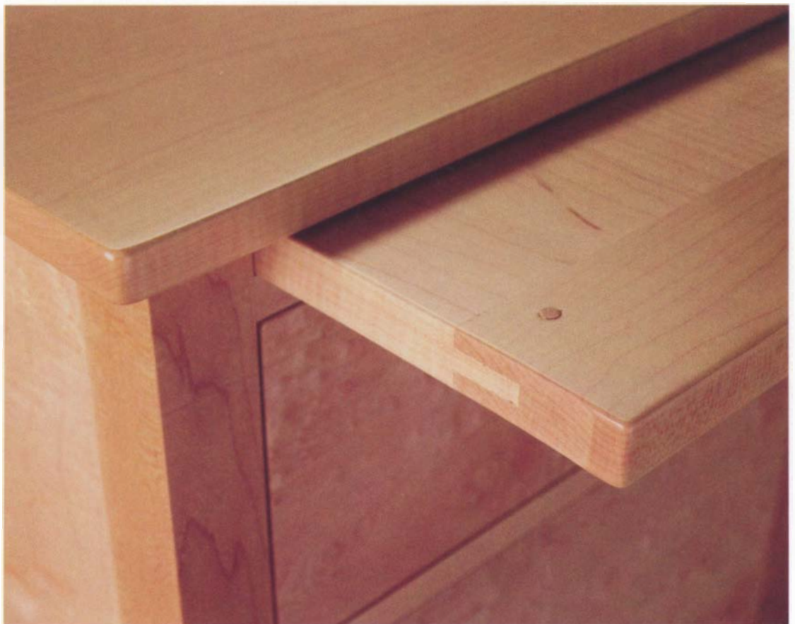
Photo G: The front edge of the pull-out board is feathered back with a sander to maintain a tight fit at the front while allowing for cross-grain expansion and contraction of the board inside the case.
