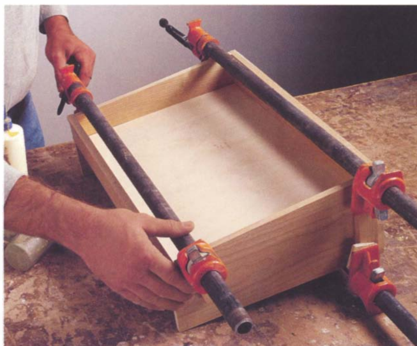
Photo F: If your dovetails fit properly, you should need to clamp the box in only one direction.
