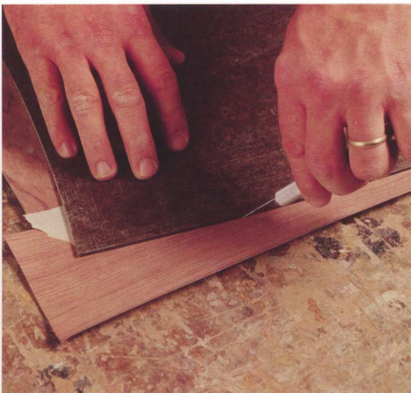
Photo H: Use a hardboard template to trim the top veneer assembly to shape.
