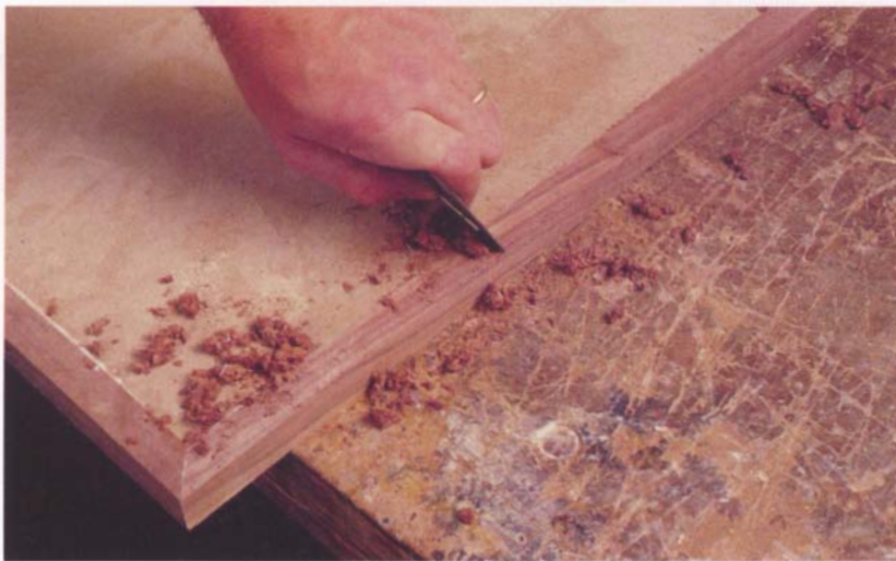
Photo F: A scraper does a good job of leveling the fall-flap panel edging.
