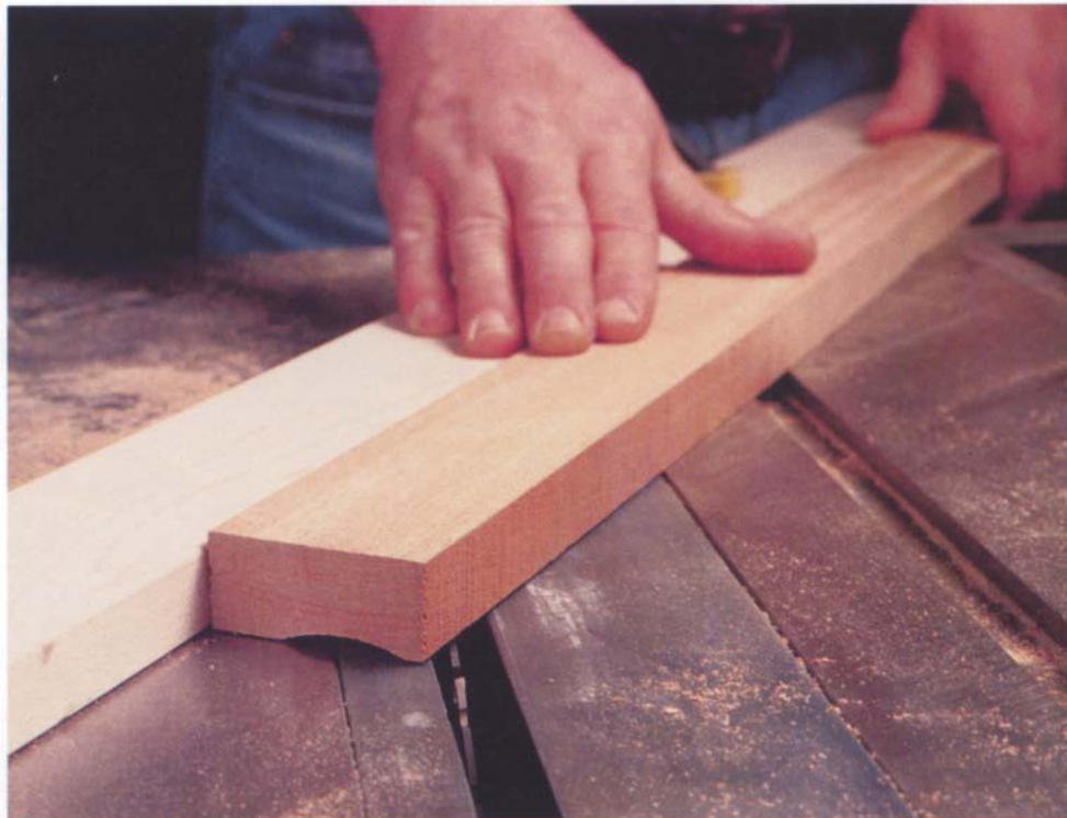
Photo D: You can cut a cove on the table saw by feeding the workpiece at an angle to the blade, taking a series of light passes.
