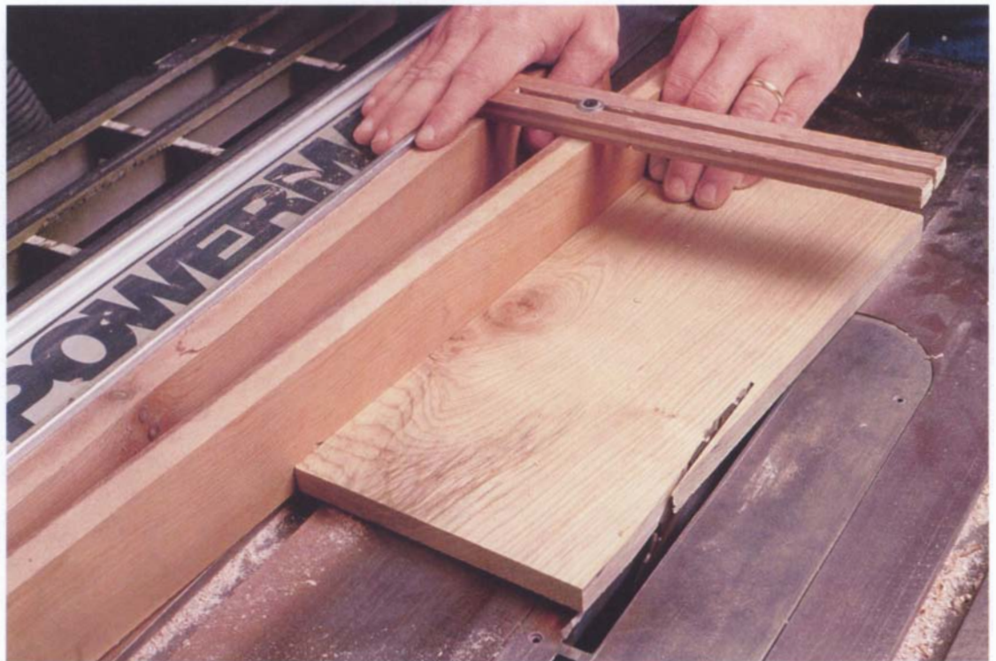
Photo A: A tapering jig allows you to cut straight, consistently accurate tapers, such as those needed on the box sides.
