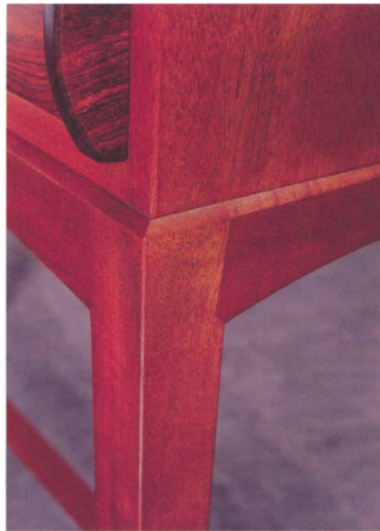
Photo A: The lower shoulder on this double-mitered leg joint avoids the weak, short-grain tip common on curved rails.
