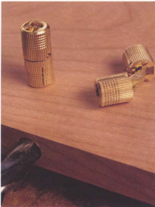
Photo E: Use a 14-mm-diameter bit to drill the holes for the barrel hinge mortises.
