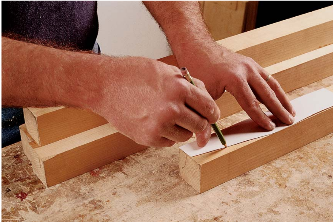
Photo B: A stiff pattern ensures that the taper on each leg will be uniform.
