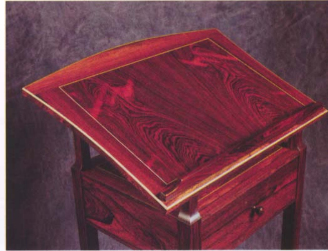
Photo E: The book-matched field on the top is set off from the border pieces with a thin framework of maple string inlay. Strips of 1/8-in.-wide maple binding wrap around the outer edges of the top.
