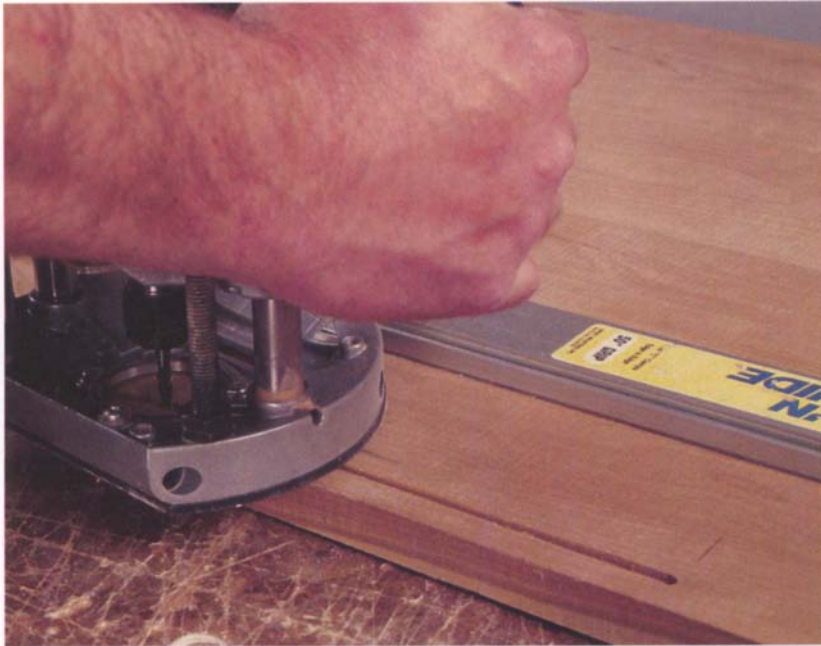
Photo D: A straight-edge and a router are used to cut the groove for the ledge in the case top.
