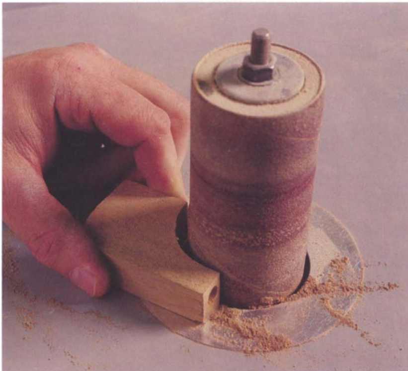
Photo H: An oscillating spindle sander is ideal for shaping inside curves, but a drum sander chucked in a drill press would also work.
