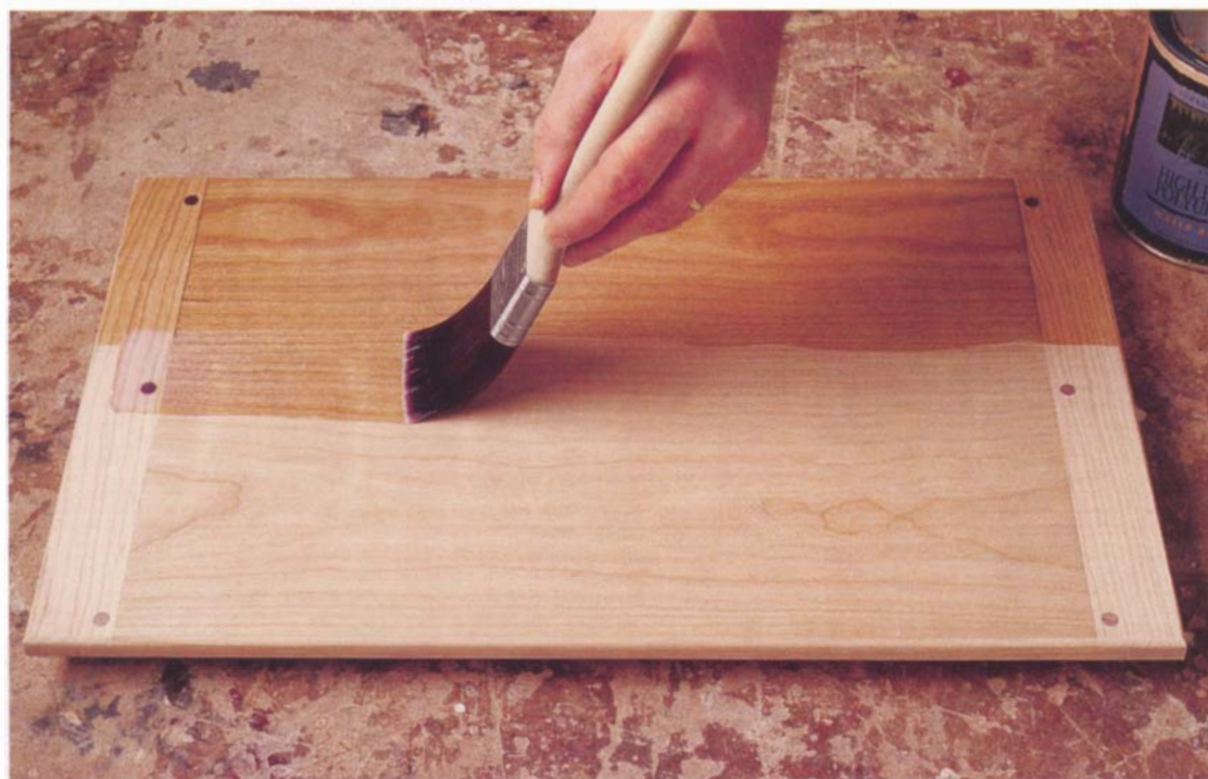
Photo J: A water-based polyurethane provides good water and abrasion resistance.
