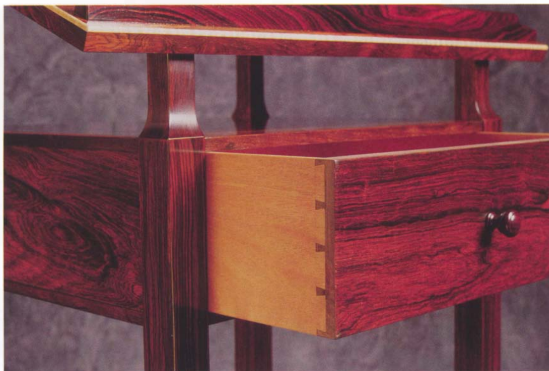
Photo K: The sides, back, and bottom of this drawer are solid mahogany. The drawer front is walnut faced with a rosewood veneer.
