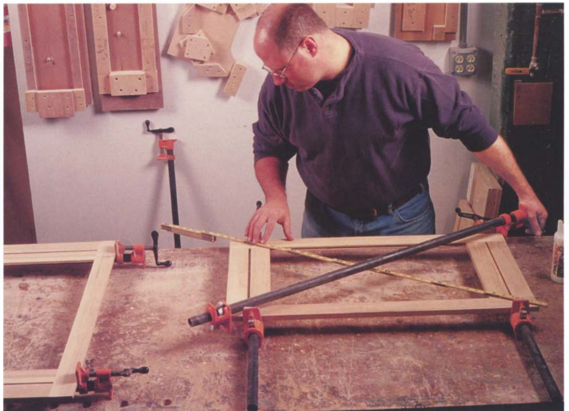
Photo G: To pull a freshly glued assembly into square, squeeze a clamp across opposite corners until opposing diagonal measurements match.
