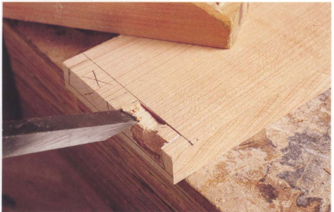
Photo 1: When removing waste between half-blind pins, make the first cuts around the perimeter of the tail socket and then work down from the top. This will prevent tearout around the sides and bottom of the joint.
