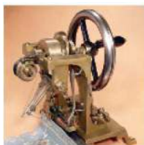
Above, from left to right: Elias Howe's patent model, using an eye-pointed needle and a shuttle to form a lock-stitch (Getty Images); Early model of Singer sewing machine (Harris & Ewing Collection, Library of Congress, Prints and Photographs Division);
