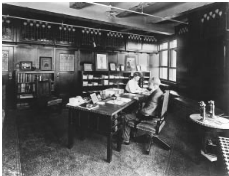
Figure 3.7 Office Telephone. By 1904, when this photograph was taken, telephones were a common feature in business offices. But, as this photograph reveals, some businessmen continued to prefer to mount them on separate tables, rather than on their desk. Note that the telephone has two transmitters. This made it possible for a stenographer to record the conversation. Telephone service quickly spread to private residences and, by the First World War, was widely available throughout the United States. Courtesy of AT&T Archives.
