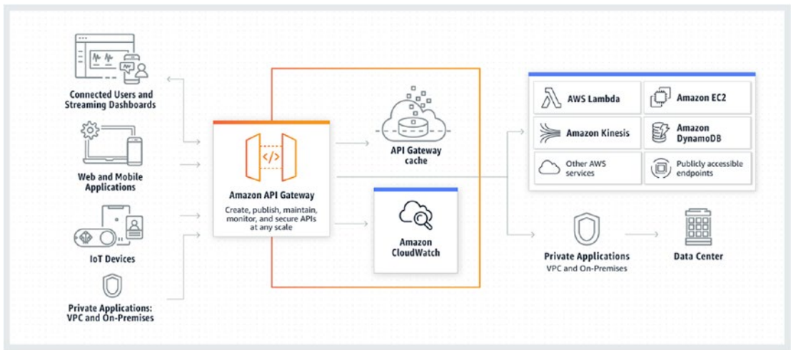
Figure 1-10. Architecture of API Gateway
