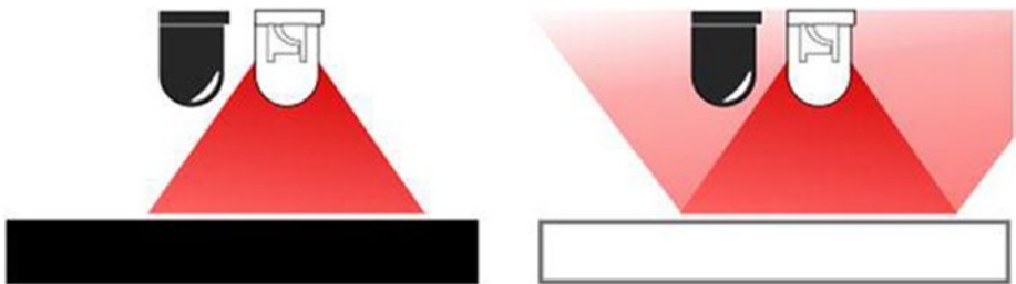
Figure 8-2. Lines and edges can be detected by the difference in reflected light
