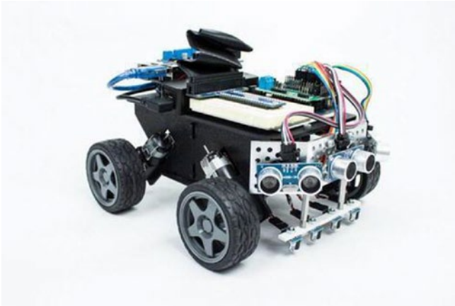
Figure 1-3. The front of our robot shows the ultrasonic sensors and Pi T-Cobbler on a breadboard
