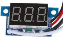
Figure 18-14 illustrates current measurement with a multimeter and by an ammeter with an LED display. In both cases, the meter is inserted in series with the load, although the circuit layout with the shunt resistor and the operational amplifier in Figure 18-13 is not as obvious. The ammeter with an LED display has a  $0.05\ \Omega$  (R050) shunt resistor and is externally powered.
