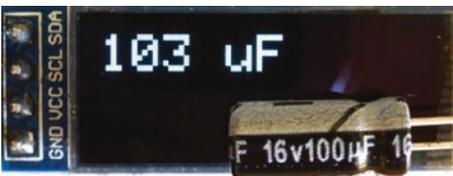
The capacitance of a capacitor is measured from the charging time of the capacitor. When a resistor,  $R$ , is connected in series with a capacitor,  $C$ , the capacitor will charge through
