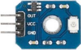
The sketch in Listing 20-2 saves the ultraviolet sensor reading to EEPROM every five seconds and displays the saved data on the Serial Monitor. The number of records is obtained with the instruction `EEPROM.get(0, records)`, rather than
