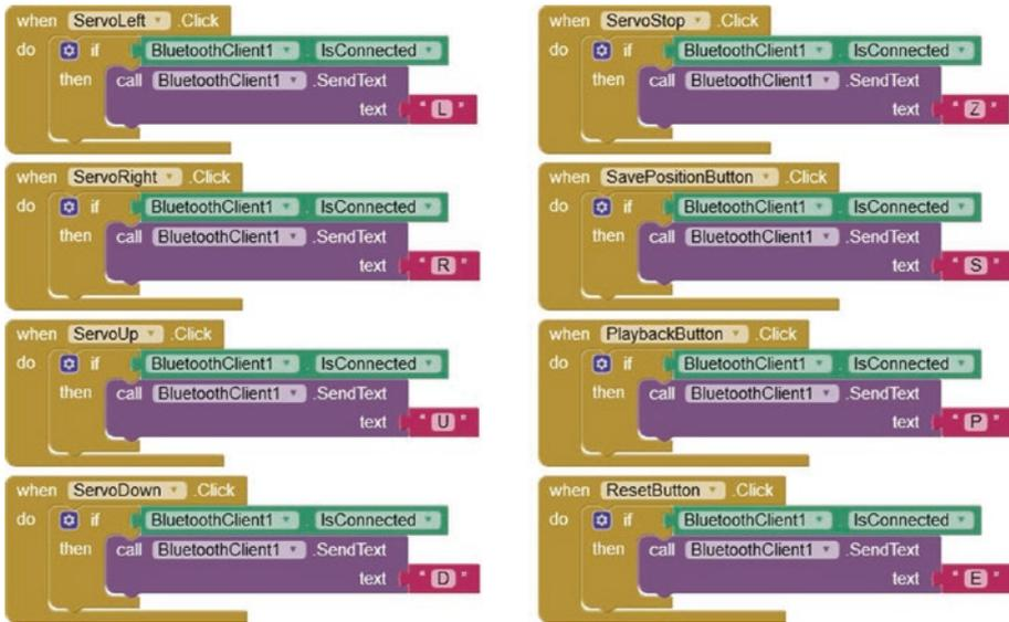
**Figure 10-14.** Servo motor commands
