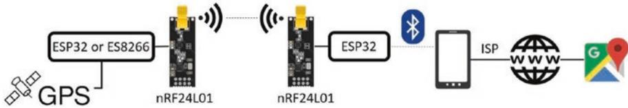
**Figure 12-1.** GPS tracking app with nRF24L01 transceiver modules
