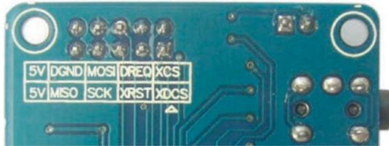
**Figure 1-2.** VS1053 connections
