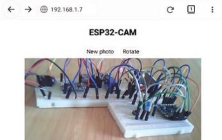
A photo taken by the ESP32-CAM module is uploaded to a web page using an HTTP request. Once the Wi-Fi connection is made and the WLAN web page loaded, clicking the *New photo* button calls the *newPhoto* function, which initiates a client HTTP request with the
