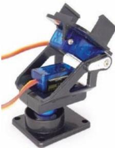
A remotely positioned laser mounted on a pan and tilt bracket, which is rotated by two servo motors, is controlled by transmitting a message containing the joystick position and the laser state. A joystick, such as the KY-023 module, consists of two potentiometers for controlling the left-right direction (X-axis) and the
