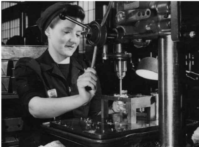
One of many wartime female factory workers using a drill press to assemble parts for use in aircrafts. [Courtesy Westport Public Library]
