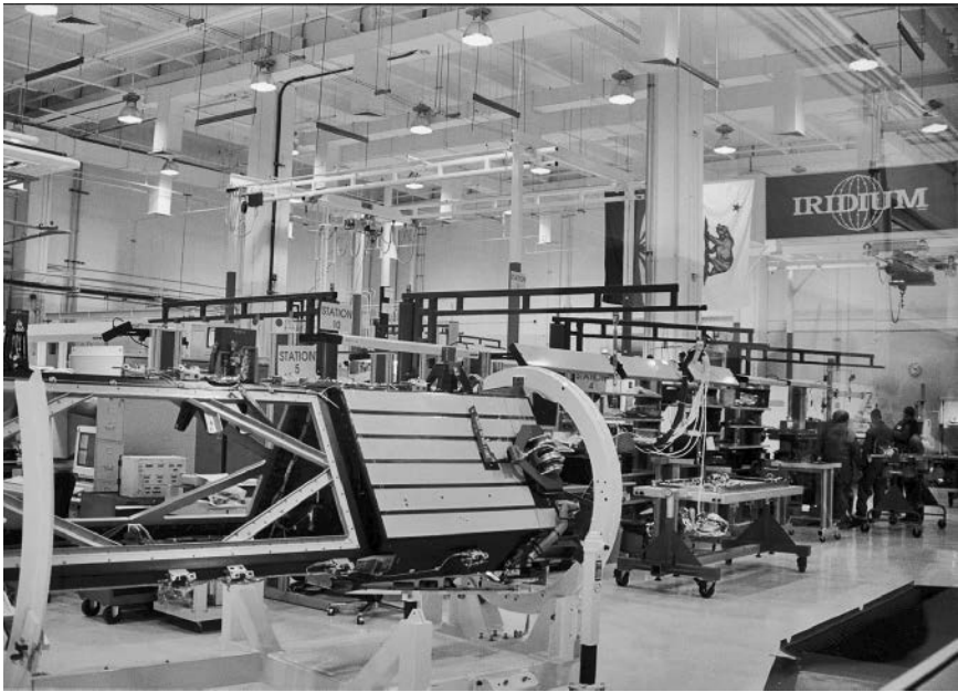
Figure 2.5. This is the basic satellite bus structure. Note the two apertures, providing openings for workers to install interior components. The white circular structure is part of the moveable dolly on which the satellite bus rests; it could be rotated to facilitate installation of interior and exterior components. Note, too, the various station signs in the assembly factory, indicating the different, sequential steps of integrating the satellite as well as the testing regimen to verify its readiness for flight. Used with permission of Motorola Solutions, Inc.
