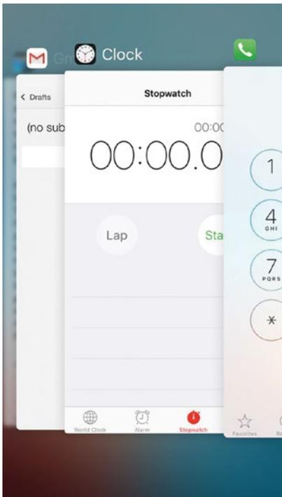
**Figure 3-5.** The iPhone multitasking screen can be quite busy with “open” apps, but few of them are using any system resources
