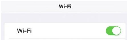
**Figure 2-1.** Toggling the Wi-Fi switch off and then on again can often solve Wi-Fi woes
