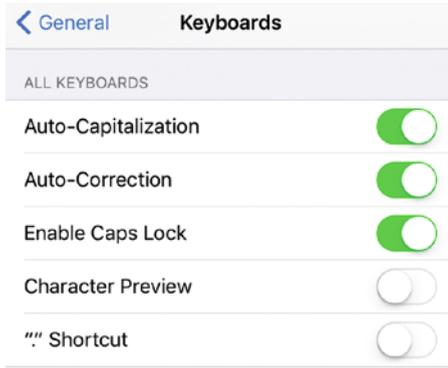
**Figure 12-4.** To type two spaces without getting a period (.), tap the "." Shortcut switch to Off
