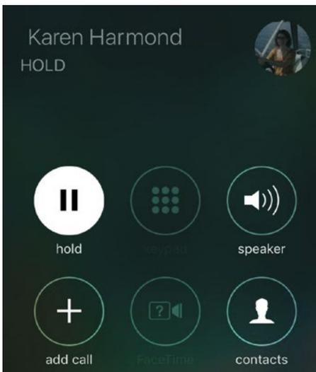
**Figure 6-10.** To put a phone call on hold, tap and hold the mute button for several seconds until you see the hold icon
