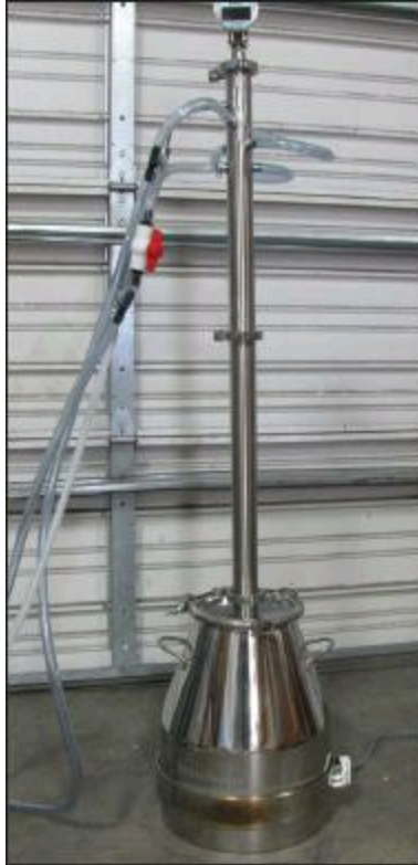
A reflux distiller with a band heater and end cap with a digital thermometer.
