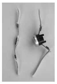
Thermal fuse (left) and thermostat (right)
