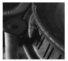
A spark jumps from an electronic igniter to the burner
