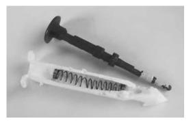
indicator. This disposable timer was made by the Heuck Company; it probably uses a different set of materials for the fusible latch than what's described in the original patent.
