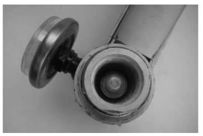
Inside view: pressure gauge (left) and valve (center)
