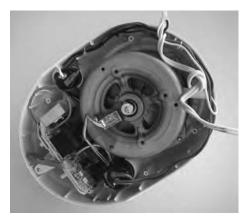
touched both at the same time. If a charge remains, you will see or hear a spark. Subsequent touches should not elicit any discharge. Now that you're held in terror by the prospect of being shocked by a vengeful capacitor, keep in mind that an old, discarded food processor will rarely have fully charged capacitors. You should still check, but as long as you make sure they're fully discharged, you will be safe.
