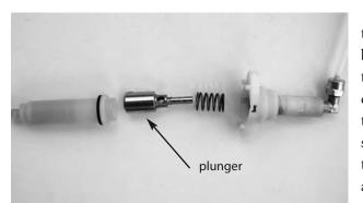
As the water is forced out of the pump, it pushes a tiny plastic ball away from the mouth of the tube. When the plunger changes direction again, a spring pushes the plastic ball back into position, sealing the mouth of the tube. In this way, it serves as a check valve, allowing water to be pumped out of the tube but preventing it from flowing back in. O-rings form seals between components to maintain the pressure.
