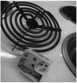
Heating coil and infinite switch
