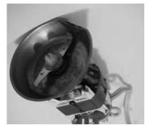
Motor and grinding blade
