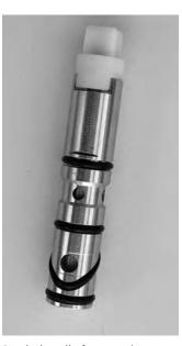
Water from one or both sources flows up through the center of the inner piece, out the smaller holes (only one is clearly visible in this picture, but there are four in all), and into the spigot.
