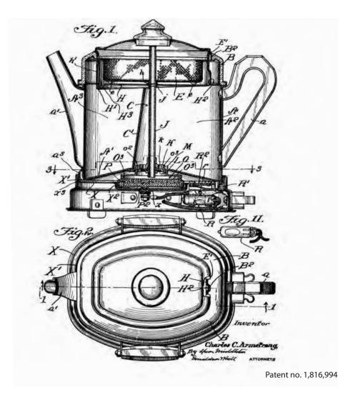
the reservoir. When the water/coffee in the reservoir has been heated to the right temperature, the thermostat cuts power to the heating coil and turns on the ready light, telling you to grab a cup.
