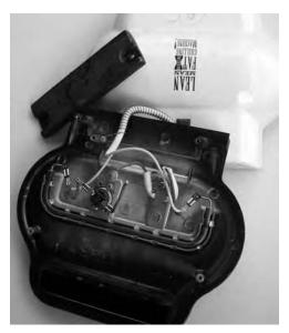
ues on into the lower section's heating element, and then into the upper heating element. A circuit in parallel to the upper heating element powers the small indicator light.
